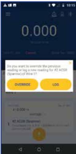
Select 'Log' to record new reading or select override to override the last reading.
