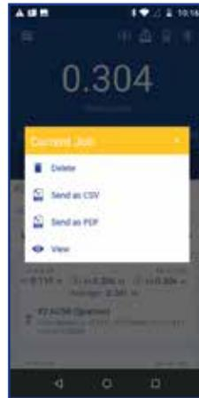
After three sets of readings have been taken for all wire ropes, a pop-up message appears to confirm 'End Weighing', once pressed, the app will display the total weight data via another pop-up. After submitting, the user has the option to view, send or delete the log; the popup will also give the user an opportunity to start a new Datalog job from there.
