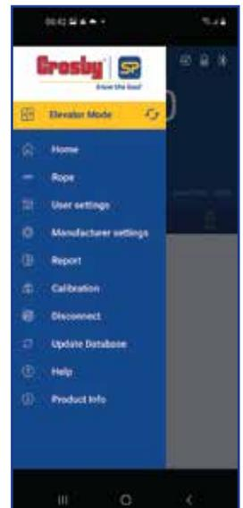
When Elevator Mode is selected – it will need activation. Tap ‘🔗’ icon to mail Straightpoint with device ID. Once received, enter the verification code to activate the elevator mode. There is also a simulation mode available in the verification code screen to check and get a feel about the mode but is not for actual use.
